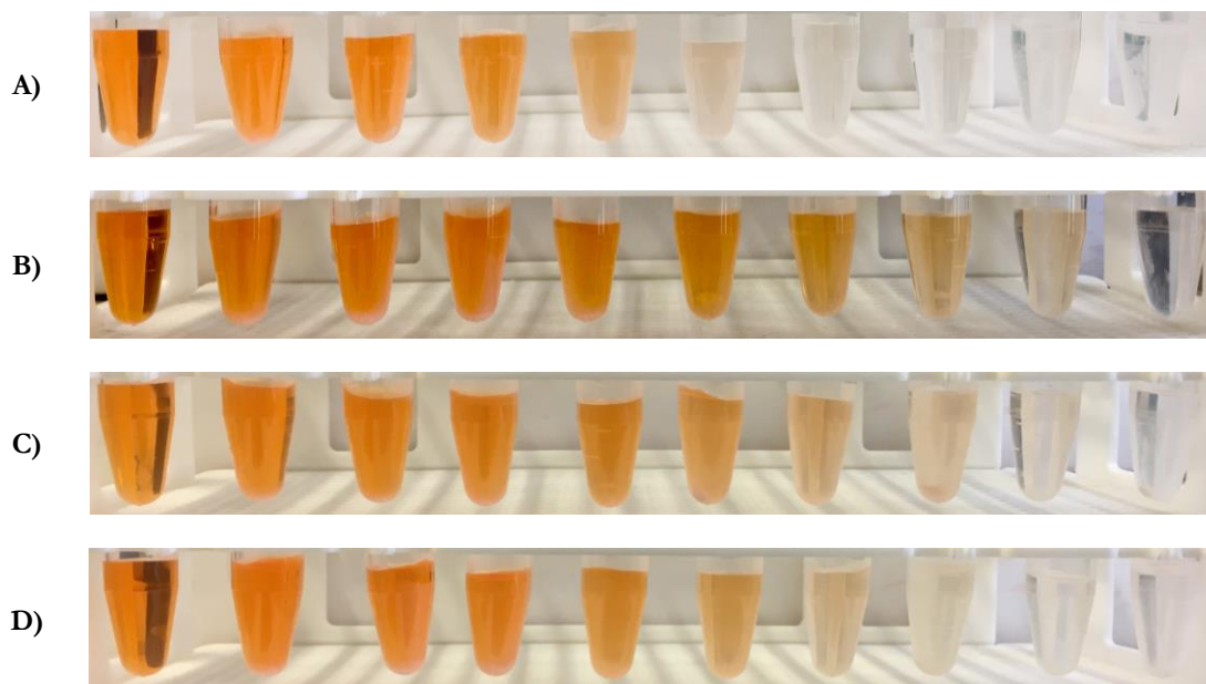
Fig. 4-4. Decolorization samples of Orange PX-2R dye with different UV-sources. A) lamp, B) square array, C) radial array, D) square&radial array.
