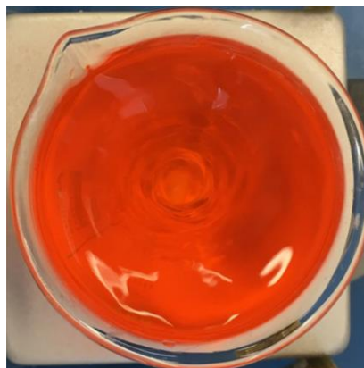
Fig. 3-15. Vortex generated by magnetic stirring. A) front view, B) Top view.
