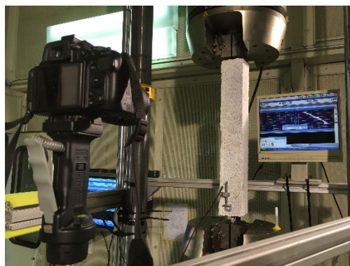
Figure 2. Experimental setup with photo camera set to take pictures at regular intervals.
