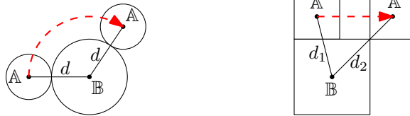
Figure 3.1: For disc robots, as \mathbb{A} slides in contact with the boundary of \mathbb{B} , the distance between their centers stays invariable. For square robots the distance between their centers changes.
