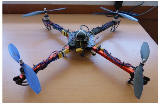
Figure 7. Quadrotor in \times configuration whose model parameters were estimated using the proposed method.
