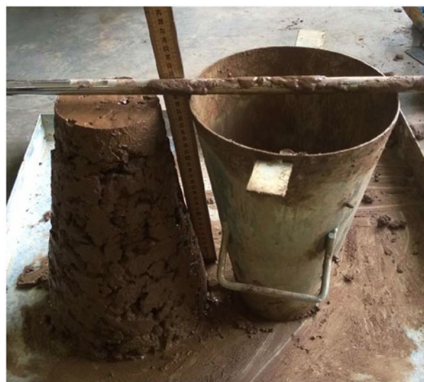
Figure 4. Determination of the slump of a fresh concrete.
