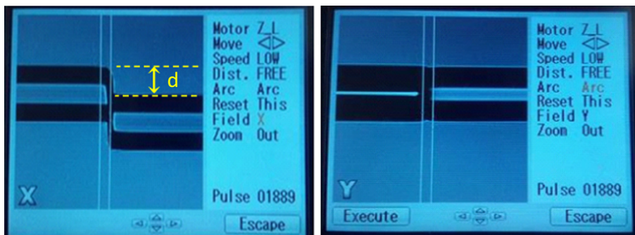
Fig. 4. Recorded image from splicing machine showing an offset splicing between two CSFs from x-direction (left) and y-direction (right).
