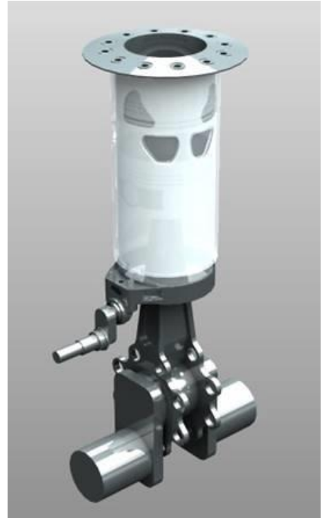
Fig. 3: CAD model of the crankshaft and a cylinder set from the Bristol Centaurus aero engine which used Burt-McCollum sleeve valves for gas exchange. Reproduced from [17].
