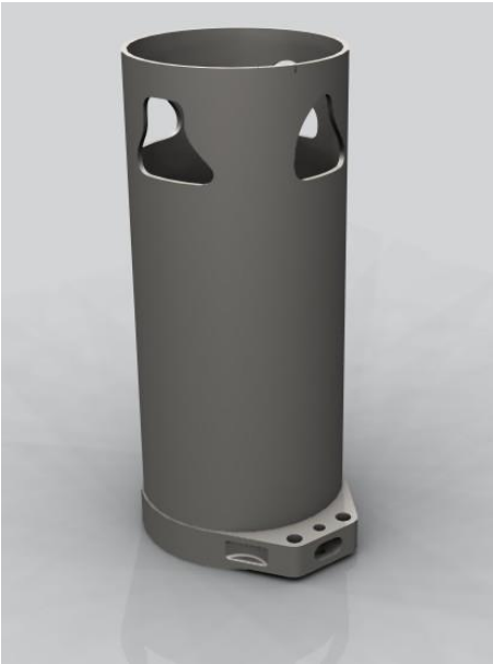
Fig. 1: CAD model of Burt-McCollum sleeve as used in the Bristol Centaurus aero engine. Reproduced from [17].
