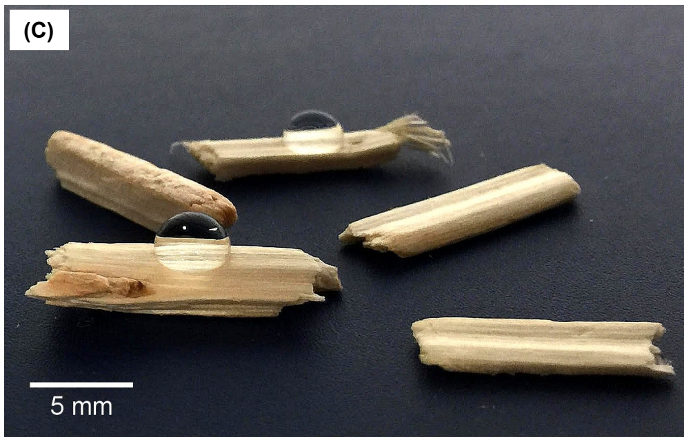
Figure 1. 3D structure of a (A) TEOS molecule, (B) HDTMS molecule; and (C) water on coated hemp shiv samples.
