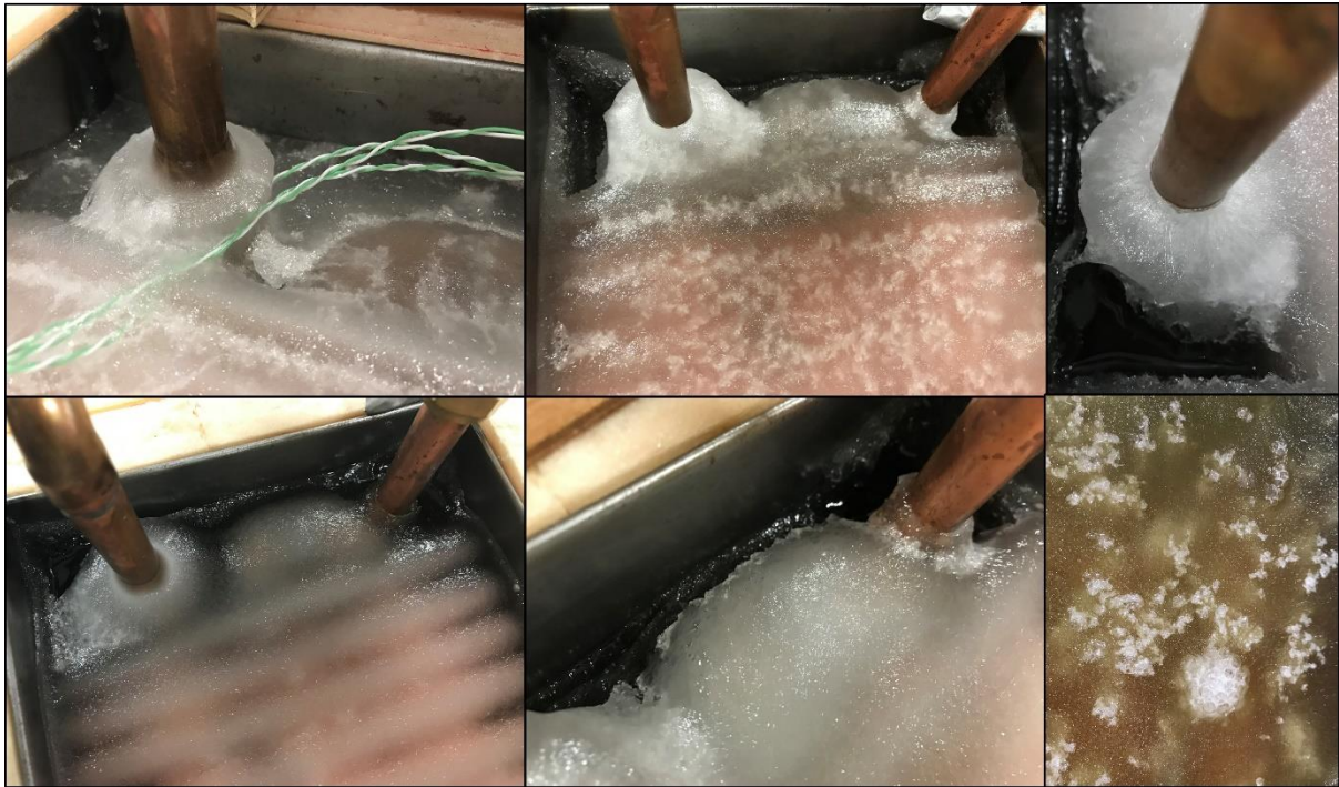
547 Figure 12: Shrinkage of volume and air bubble deposits due to ullage after PCM solidification
