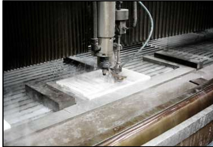
Fig. 1. Water cutting technique used to cut out the openings.
