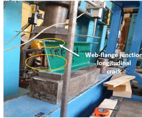
Fig. 11. Failure mode FRP-C-Co 4.
