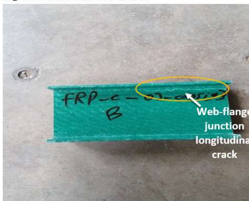
Fig. 10. Failure mode FRP-C-Co 3.
