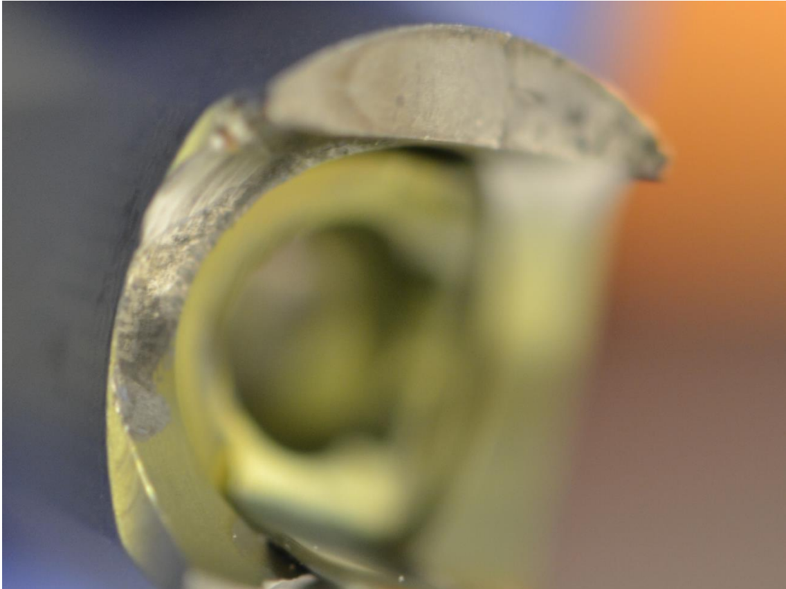
Figure 3.1.1 Close-up photo of the fracture surface.
