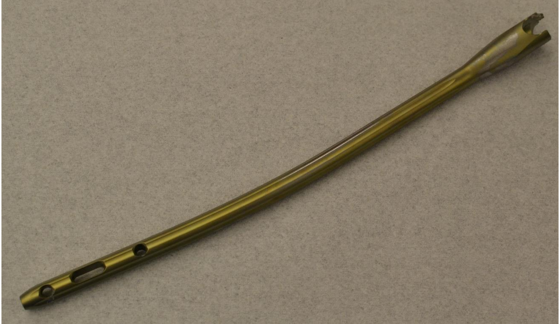
Figure 2.1.1 Distal portion of the failed nail.
