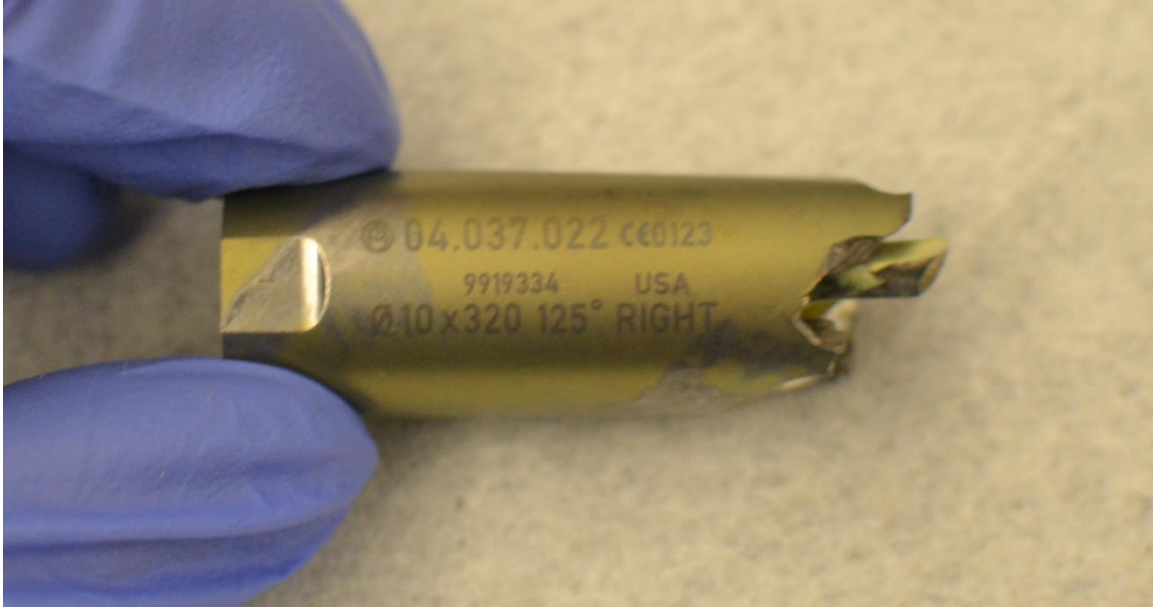
Figure 2.1.2 Proximal portion of the failed nail.
