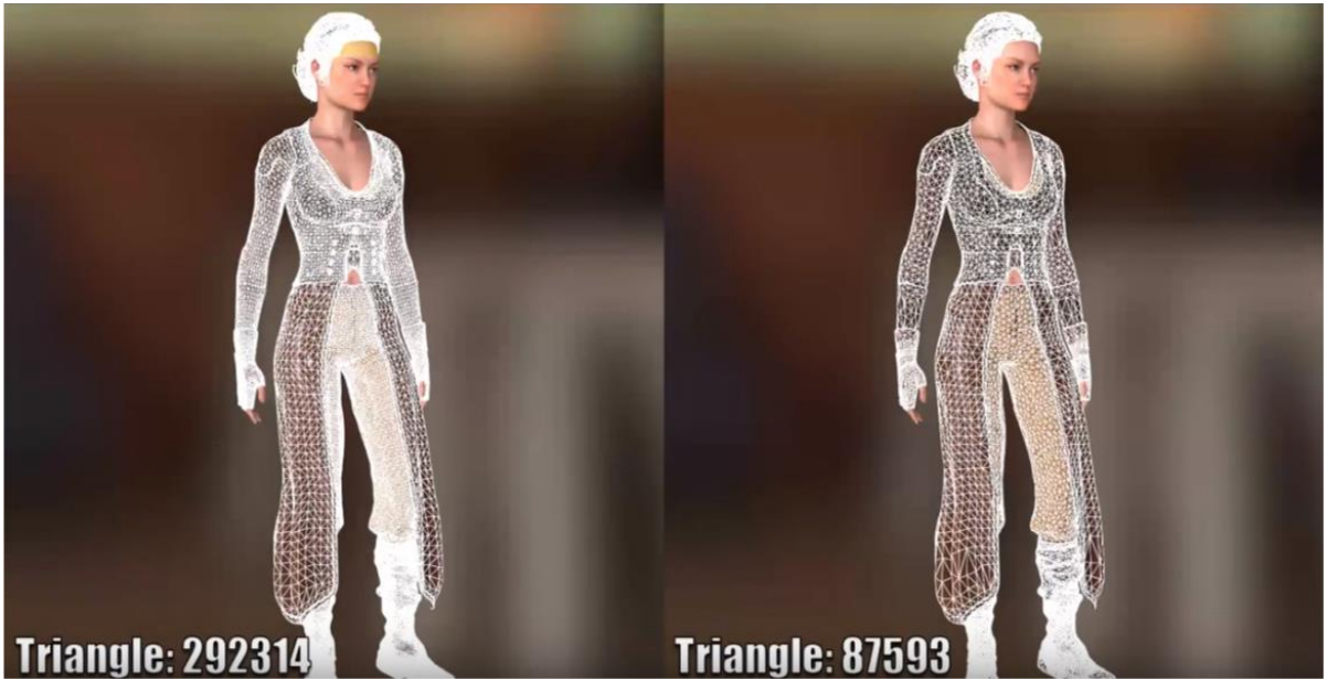
Fig 10: Reduction of polygons in the model and all its components.[11]
