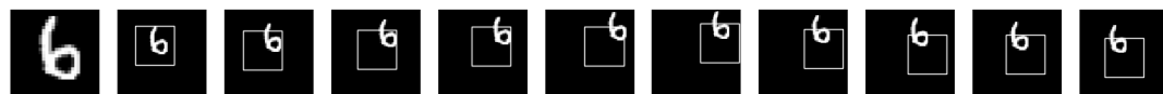
Figure 4.78: A visual representation of the GOTURN model tracking a 30 frame sequence with a handwritten digit 6. The first image in the first row represents the object the model is attempting to track. Two frames were skipped between each.
