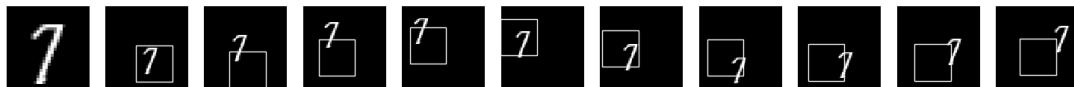
Figure 4.79: A visual representation of the GOTURN model tracking a 30 frame sequence with a handwritten digit 7. The first image in the first row represents the object the model is attempting to track. Two frames were skipped between each.
