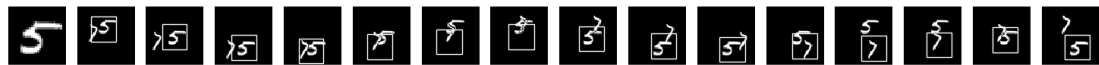
Figure 4.62: A visual representation of C-DATM tracking a 30 frame sequence with handwritten digits 5 and 7. The first image in the first row represents the object the model is attempting to track. A frame was skipped between each.
