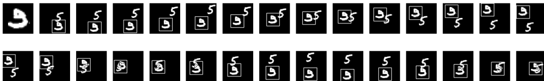
Figure 4.138: A visual representation of C-DATM trained with a mixture of 1 and 2-digit training data, tracking a 30 frame sequence with handwritten digits 3 and 5. The first row is the first 14 images in the sequence, excluding the first frame, and the second row is the last 15. The first image in the first row represents the object the model is attempting to track.
