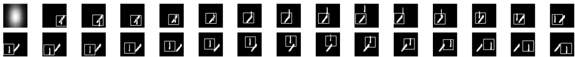
Figure 4.103: A visual representation of C-DATM tracking a 30 frame sequence with handwritten digits 1 and 1. The first image in the first row represents the object the model is attempting to track. A Gaussian blur rate of 5 was applied to the condition.
