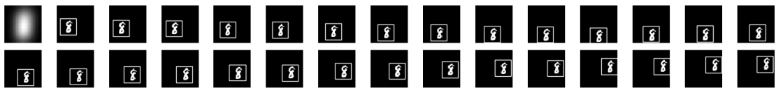
Figure 4.92: A visual representation of C-DATM tracking a 30 frame sequence with a handwritten digit 8. The first image in the first row represents the object the model is attempting to track. A Gaussian blur rate of 4 was applied to the condition.
