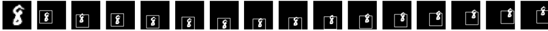
Figure 4.65: A visual representation of the GOTURN model tracking a 30 frame sequence with a handwritten digit 8. The first image in the first row represents the object the model is attempting to track. A frame was skipped between each.
