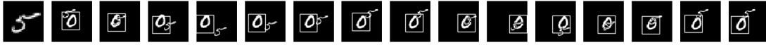
Figure 4.64: A visual representation of C-DATM tracking a 30 frame sequence with handwritten digits 5 and 0. The first image in the first row represents the object the model is attempting to track. A frame was skipped between each.
