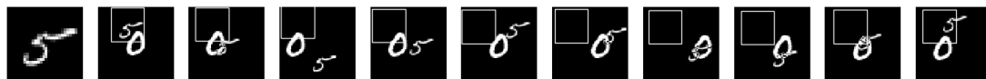
Figure 4.82: A visual representation of the GOTURN model tracking a 30 frame sequence with handwritten digits 5 and 0. The first image in the first row represents the object the model is attempting to track. Two frames were skipped between each.
