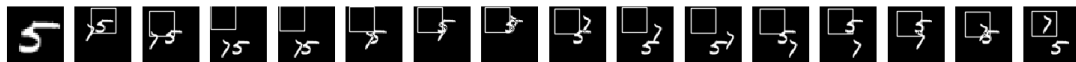
Figure 4.68: A visual representation of the GOTURN model tracking a 30 frame sequence with handwritten digits 5 and 7. The first image in the first row represents the object the model is attempting to track. A frame was skipped between each.
