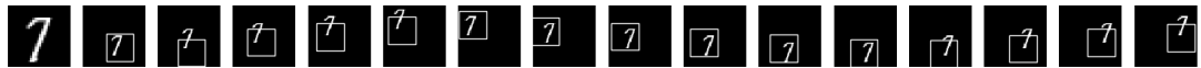
Figure 4.67: A visual representation of the GOTURN model tracking a 30 frame sequence with a handwritten digit 7. The first image in the first row represents the object the model is attempting to track. A frame was skipped between each.
