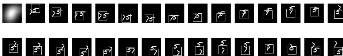
Figure 4.118: A visual representation of the GOTURN model tracking a 30 frame sequence with handwritten digits 5 and 7. The first image in the first row represents the object the model is attempting to track. A Gaussian blur rate of 5 was applied to the condition.
