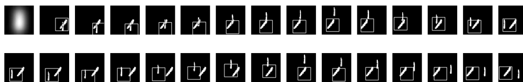
Figure 4.117: A visual representation of the GOTURN model tracking a 30 frame sequence with handwritten digits 1 and 1. The first image in the first row represents the object the model is attempting to track. A Gaussian blur rate of 4 was applied to the condition.
