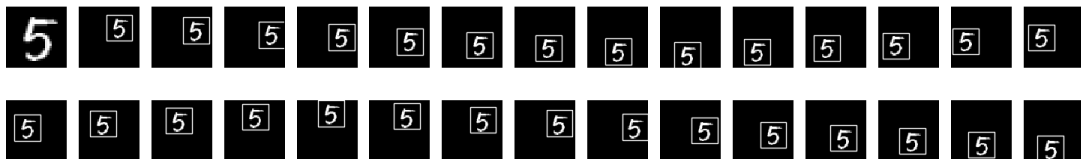
Figure 4.132: A visual representation of C-DATM trained with a mixture of 1 and 2-digit training data, tracking a 30 frame sequence with a handwritten 5 digit. The first row is the first 14 images in the sequence, excluding the first frame, and the second row is the last 15. The first image in the first row represents the object the model is attempting to track.
