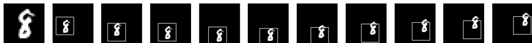
Figure 4.77: A visual representation of the GOTURN model tracking a 30 frame sequence with a handwritten digit 8. The first image in the first row represents the object the model is attempting to track. Two frames were skipped between each.
