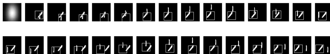
Figure 4.119: A visual representation of the GOTURN model tracking a 30 frame sequence with handwritten digits 1 and 1. The first image in the first row represents the object the model is attempting to track. A Gaussian blur rate of 5 was applied to the condition.
