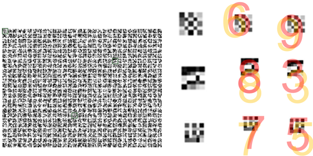
Figure 5.8: This Figure is the end-to-end trained kernels of the second dilated convolution layer in our tracker. Showing kernels representing moving edge features, with examples of 6, 9, 8, 3, 7, and 5 moving across the features.
