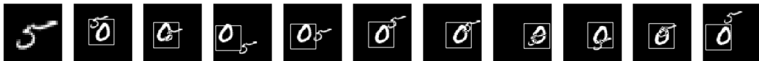
Figure 4.76: A visual representation of C-DATM tracking a 30 frame sequence with handwritten digits 5 and 0. The first image in the first row represents the object the model is attempting to track. Two frames were skipped between each.
