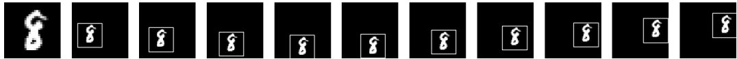
Figure 4.71: A visual representation of C-DATM tracking a 30 frame sequence with a handwritten digit 8. The first image in the first row represents the object the model is attempting to track. Two frames were skipped between each.
