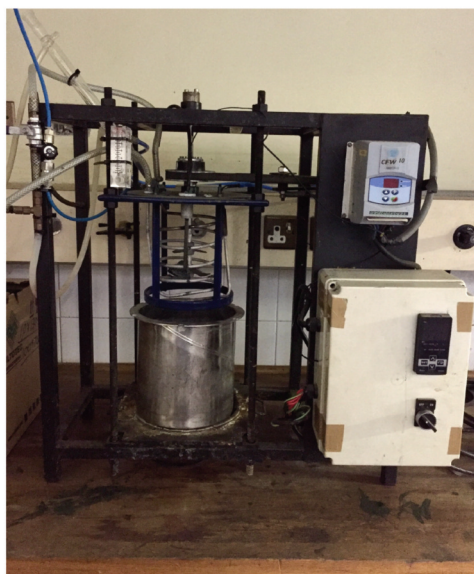
Figure 2—Schematic and photo of the laboratory atmospheric batch leaching reactor
