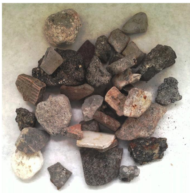
Fig. 5. Ceramic materials contained in the coarse fraction (N 16 mm). This picture was taken from a previously washed fraction.
