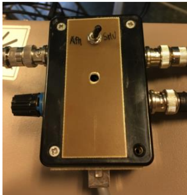
Figure 5.16 Picture of the external switch control unit where the RJ45 cable is connected. It can be seen a control switch for AFM or SMU measurements, the selector of the three transistors (bottom-left) that selects one of the three drain connections visible on the unit.
