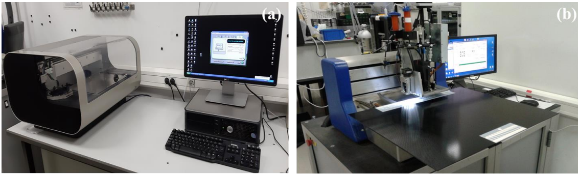
Figure 2.4 (a) Picture of Dimatix 2831 inkjet printer from Fujifilm. (b) Picture of Carnelian 4000 inkjet printer from Xennia.
