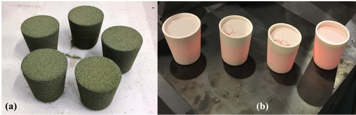
741 Figure 3: LOI test with (a) 3DP specimens, (b) immediately after taking out of the oven at 742 900 °C
