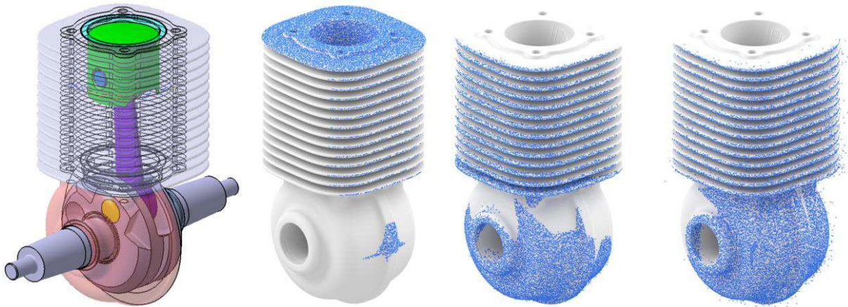
Figure 8: CAD model of a compressor reversed engineered with configurations 1 to 3.
