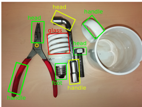
Fig. 4: Objects used for our experiment, with name of grasping locations. Green color (resp red color) denotes authorized (resp prohibited) grasping location. Yellow color is used to illustrate authorized/prohibited location and vice versa, depending on the task (for example the accessibility of the screwing operation). For the pliers, two different authorized locations are tested separately.
