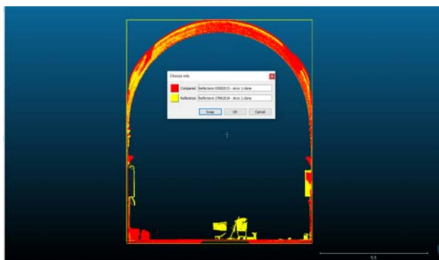
Figure 9: comparing cloud to cloud with Cloudcompare. Clouds data 2015 and 2019
