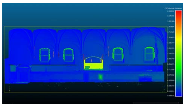
Figure 16: Cloud to cloud comparison (original state and final state) lateral east and west
