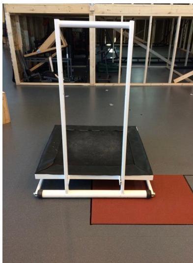
Figure 2. The trampoline was placed in the middle of the force plate with the handle in front of the subject. Subjects began behind the trampoline and then stepped on to perform the jump.
