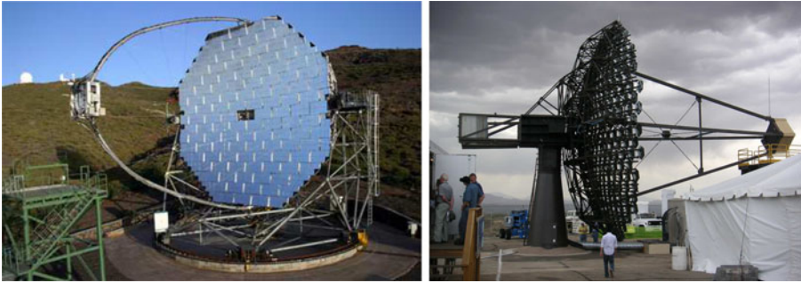
Fig. 27 Examples of alt-azimuth mount, as used for H.E.S.S. and MAGIC ( left ) and a central positioner design, used for the Whipple and VERITAS telescopes ( right )
