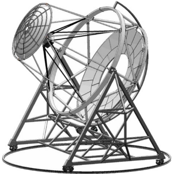
Fig. 34 Model of an AGIS Schwarzschild–Couder telescope and its two-mirror aplanatic optical system (from [96])
