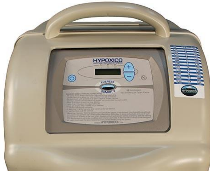
Figure 6.1: Hypoxia generator (Everest Summit II Hypoxic Generator; Hypoxico, Inc., New York, U.S. used in the study to induce hypoxia in subjects.
