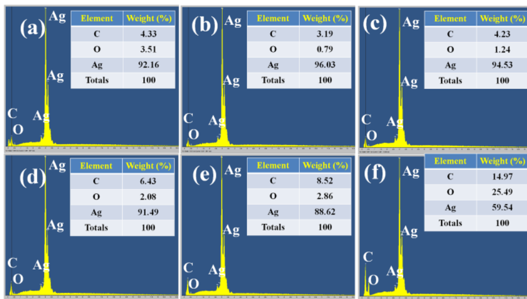
Figure 7.10 EDS results of silver films sintered at 150°C for 60min from different silver oxalate inks, (a) Ethylenediamine, (b) 1,2-diaminopropane, (c) butylamine, (d) hexylamine, (e) octylamine, (f) ethanolamine
