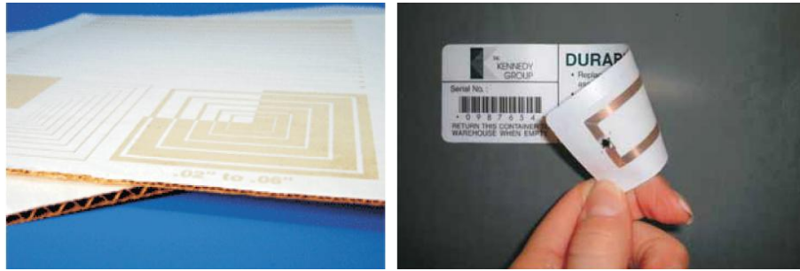
Figure 2.1 (a) An RF antenna printed onto corrugated stock; (b) A printed RFID Tag [66]
