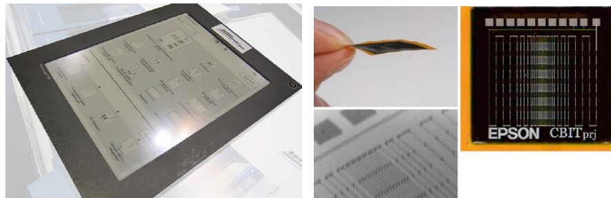
Figure 2.2 (a) A4-sized e-book with a printed back plane (Courtesy of Plastic Logic, Cambridge, UK); (b) Flexible 20 layers wiring printed circuit board (PCB) made with inkjet printing (Courtesy of EPSON, Nagano, Japan) [68]
