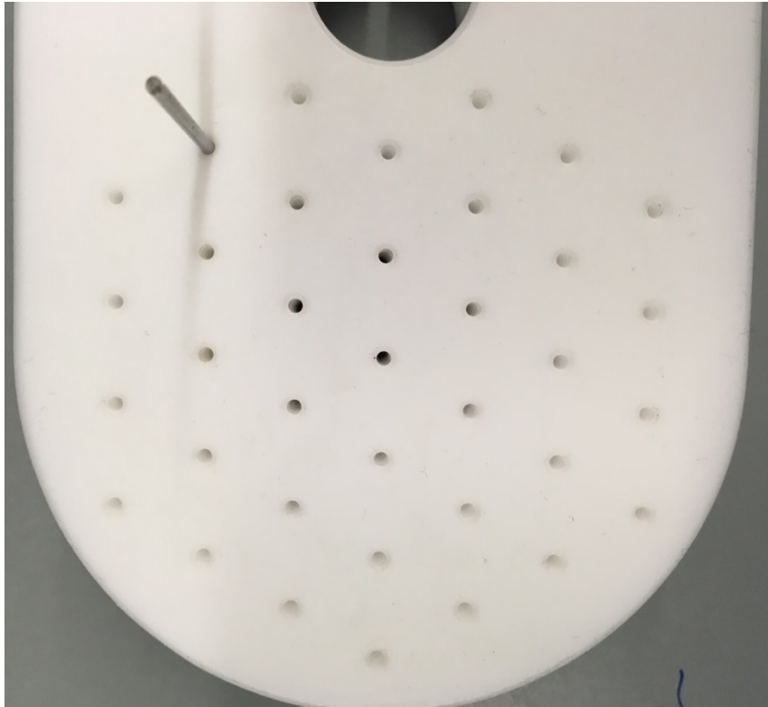
Figure 24. Multi-point inoculator. Individual inoculating pins (delivering approximately 1 \mu l spot of inoculum onto agar) are arranged into the existing holes.
