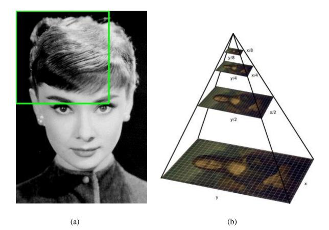
Figure 4. Example to window sliding (a) and pyramid of the image (b) [61]
