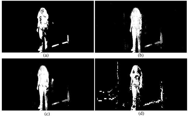
Figure 13. OpenCV Backgraund Subtraction methods: (a) BackgroundSubtractorMOG; (b) BackgroundSubtractorMOG2; (c) BackgroundSubtractorKNN; (d) BackgroundSubtractor-GMG;
