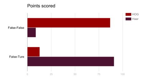
Figure 17. Comparison of HOG and Haar based human detection methods on 100 False images. False-False - where False images (non-human images) do not have detection; False-True - when False images (nonhuman images) are detected.
