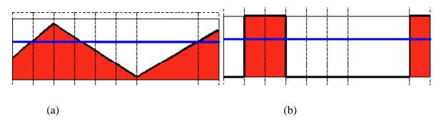
Figure 6. Thresholding process: (a) an original image. (b) a binary image
