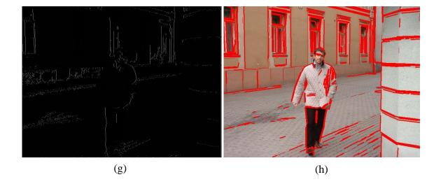
Figure 8. Feature detection methods: (a) SIFT; (b) SURF; (c) LoG (Laplacian of Guassian); (d) Harris operation, (e) Canny, (f) HOG, (g) Contour feratures, (h) Line Segment Detector
