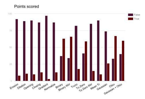
Figure 11. Detection results with pre-processing methods on False images
