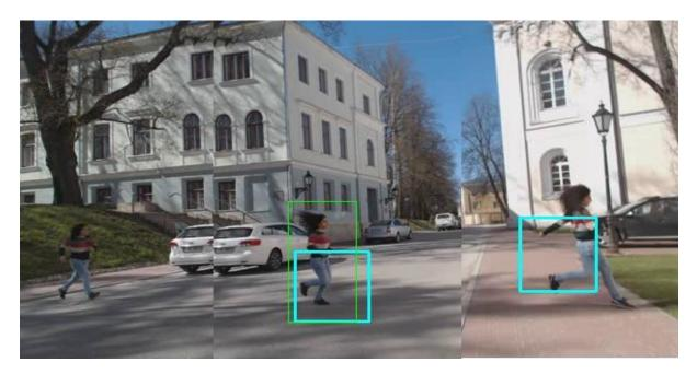
Figure 19. The second pedestrian detection and tracking approach. Here the blue rectangle is a tracker, green rectangle is a detector.
