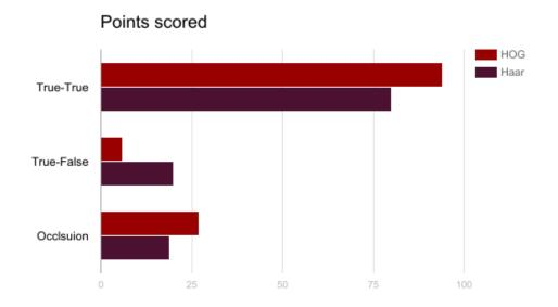
Figure 16. Comparison of HOG and Haar based human detection methods on 100 True images True-True is a True detection on True images (human images); True-False is a False detection on True images (human images).
