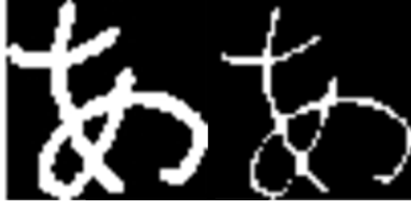
Figure 4. On the left input image for erosion, on the right output of erosion
