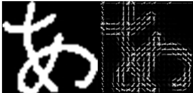
Figure 9. Input image on the left and extracted and visualized HOG feature on the right
