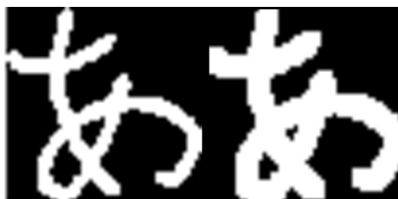
Figure 6. On the left input image for dilation, on the right output of dilation
