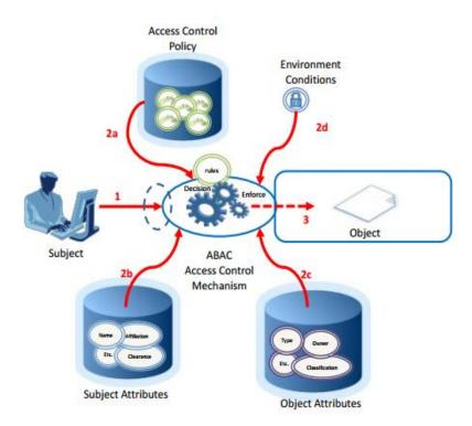
Figure 8: ABAC Basic Mechanism [16]
