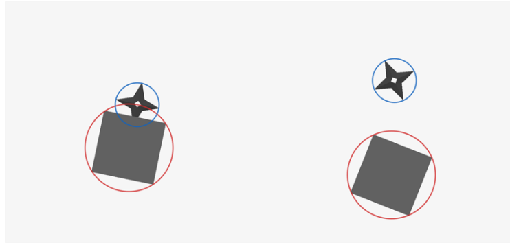
Illustration 15. The bounding circles of the shuriken and a platform intersecting on the left and not intersecting on the right of the illustration.
