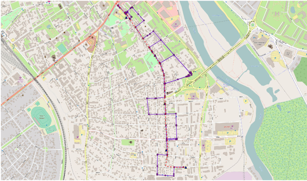
Figure 8: Trajectory reconstruction based on CDR data. GPS trajectory is in red and CDR trajectory is in blue.
