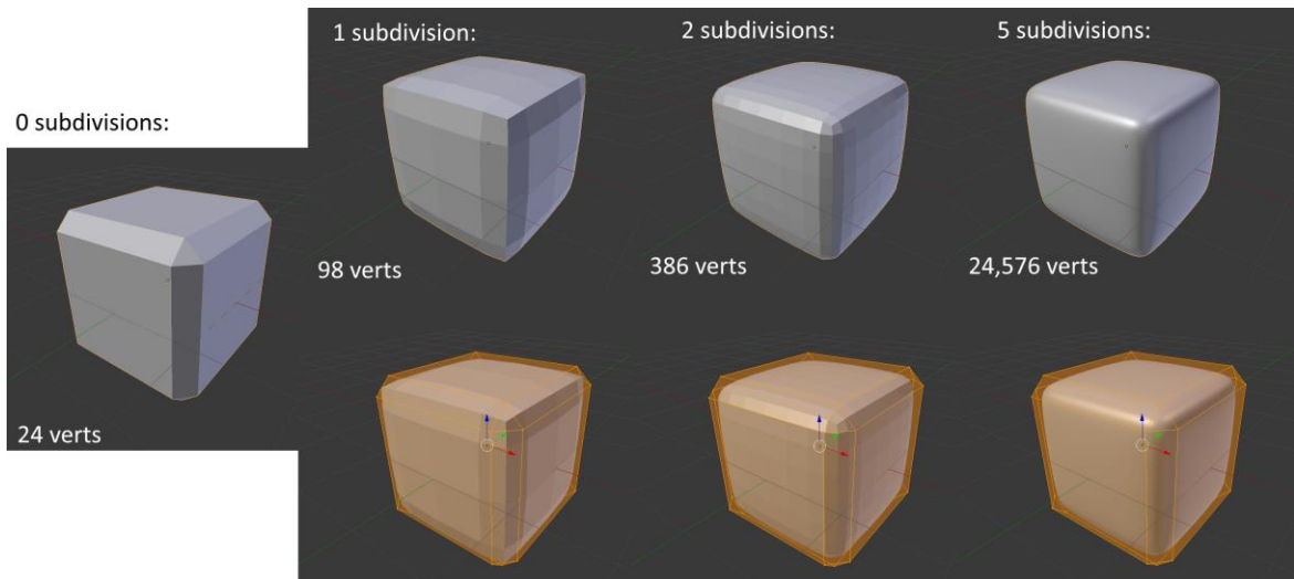
Figure 26. A beveled cube in Blender subdivided with Catmull-Clark subdivision algorithm after 0, 1, 2, and 5 subdivisions from left to right. The vertex counts displayed are of the smooth-shaded model.
