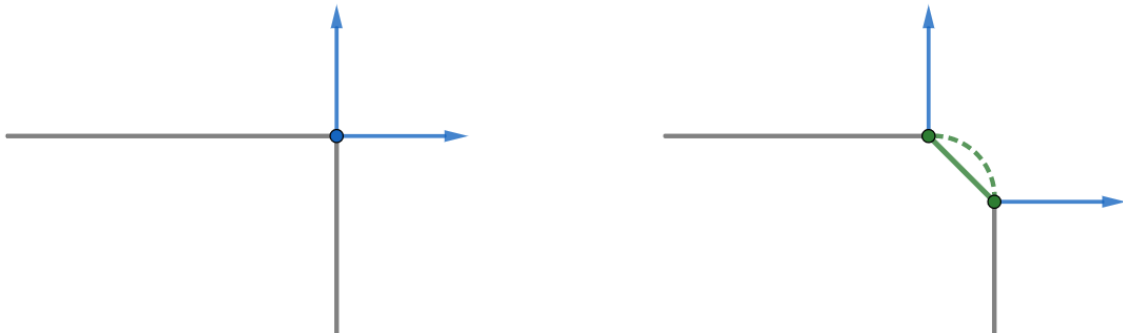
Figure 17. Normals on a hard edge before (left) and after chamfering (right).
