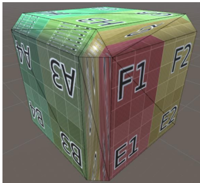
Figure 61. Seamed cube after chamfering without recreating seams corresponding to the UV map in Figure 60. Three chamfered edges are visible where the texture is mapped from a big part of the UV map.
