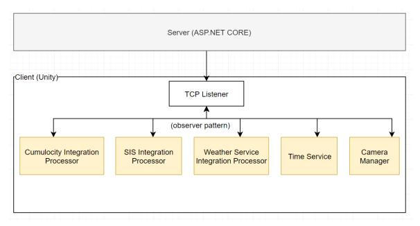
Figure 3. Components of the observer pattern: subject (white) and observers (yellow).
