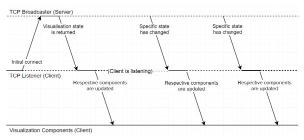
Figure 4. The communication process.
