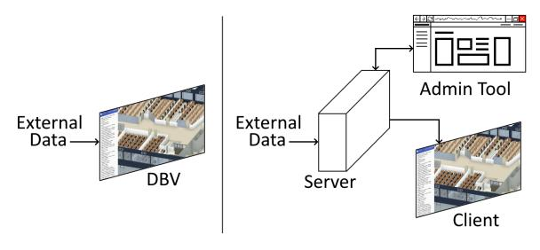
Figure 1. The old (left) and new (right) structure of the project.
