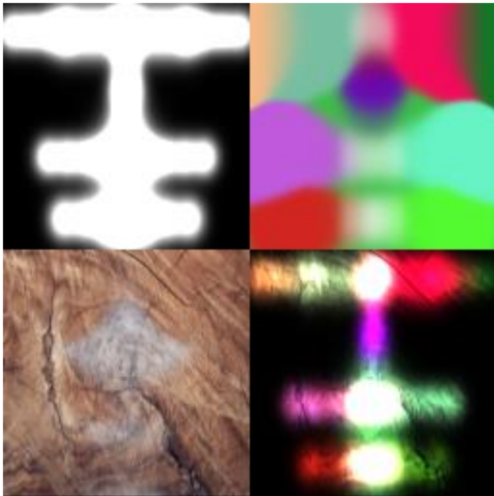
Figure 25. Example of the parts of a generated texture. Top-left is the sum. Top-right is the colour. Bottom-left is the combination of base textures. Bottom-right is the final combination of these values multiplied together.
