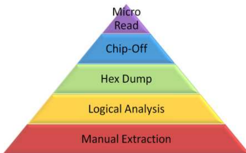
Figure 11. Sam Brothers cellular phone tool levelling pyramid [22]
