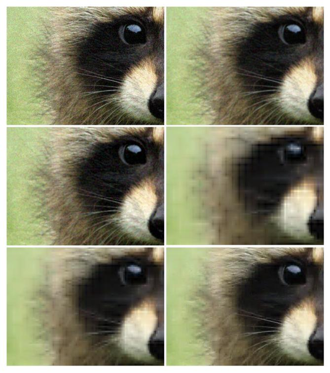
Figure 11: Quality comparison of various denoising methods on the Raccoon image. The images are row-by-row as follows: Original corrupted by Gaussian noise,  $\sigma$ =20. 3×3 mean filtered. 3×3 median filtered. Original BayesShrink, orthogonal wavelet, soft thresholding. BayesShrink, k=1.0, orthogonal wavelet, soft thresholding. BayesShrink, k=0.7, orthogonal wavelet, moderate thresholding.
