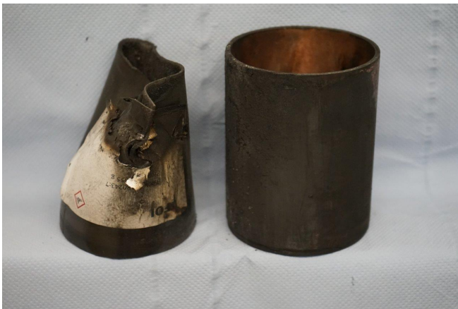
Fig. 5. Thermal insulation of the walls with carbon black insulation coat (left) and a phenolic liner (right) after usage
