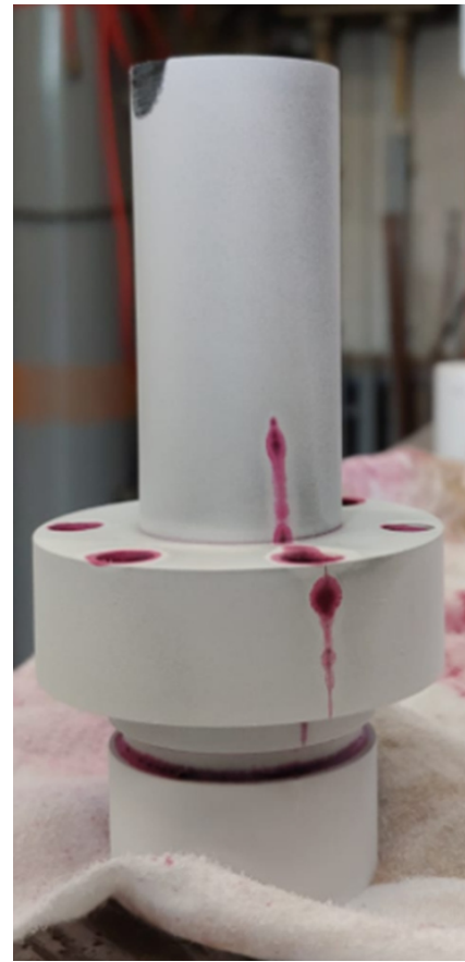
Fig. 6. Penetrant dye inspection of the tungsten nozzle
