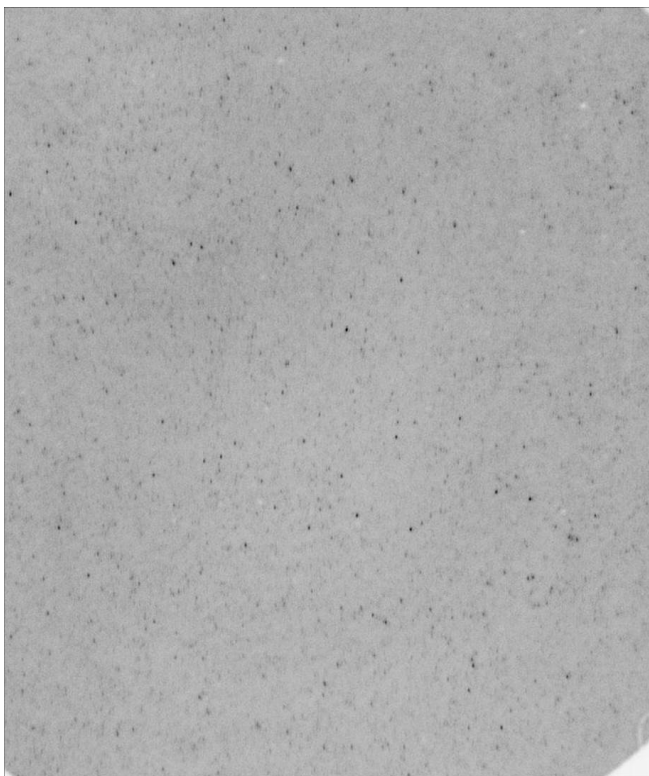
Fig. 14. Randomly selected (inverted) raw intensity images of the DIPSD measurements with the Ex3-P2 nozzle and with the HTPB0514 propellant grain (Run031-V06-End). The image/field of view corresponds to 3.4 mm × 4.0 mm.
