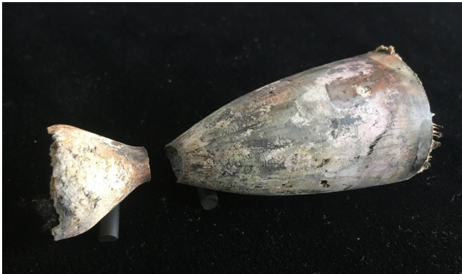
Fig. 10. Deposition of alumina in the nozzle for the propellant 5% aluminum propellants HTPB0514 (after removal from the nozzle contour)
