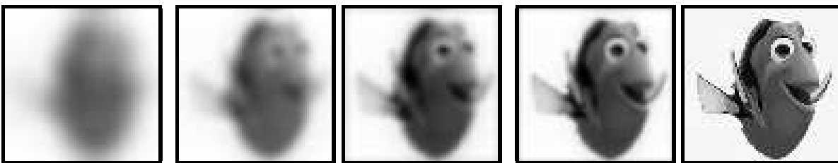
FIG. 9. Simulated comparison of images reconstructed using arrays of detectors of increasing size. Left: image reconstruction using a 5 \times 5 detector array. Second from left: image reconstruction using a 10 \times 10 detector array. Middle: Image reconstruction using a 15 \times 15 detector array. Second from right: Image reconstruction using a 26 \times 26 detector array. Right: Original image before reconstruction section F. Imaging simulation.
