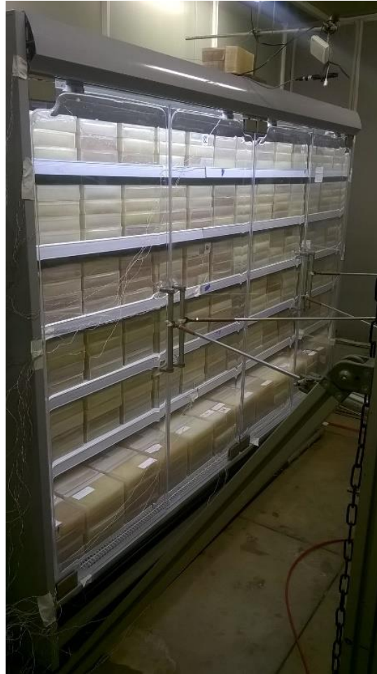
Figure 2: Cabinet with retrofitted doors.
