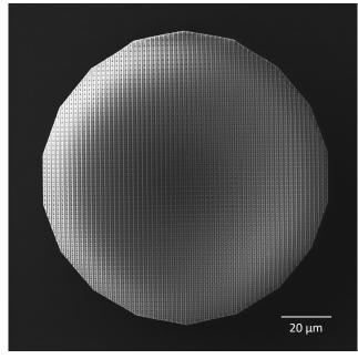
(a) Fabricated woodpile structure of a cylinder shape.
