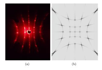
Fig. 3: (a) Laue diffraction pattern of 3D PhC woodpile structure with period  $a = 2 \ \mu m$ , irradiated by a monochromatic laser light with a wavelength  $\lambda = 635 \ nm$ . (b) Calculated diffraction pattern of woodpile structure with period  $a = 2 \ \mu m$ , irradiated by a monochromatic laser light with a wavelength  $\lambda = 633 \ nm$  [11].
