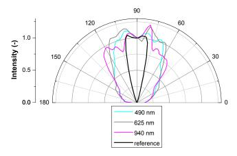
Fig. 5: <110> cross-section of far-field radiation patterns of modified multi-mode optical fiber by a 3D PhC wood-pile structure with period of 2  $\mu$ m measured at stated wavelengths.
