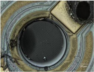
Fig. 8: Confocal image of InGaAsN-based photodiode with applied 3D PhC woodpile structure at surface.
