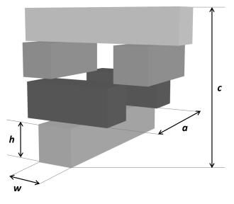
Fig. 1: The four-layer sequence arrangement of diamond-like woodpile structure [4].
