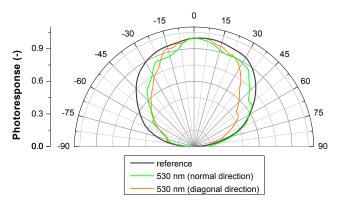
Fig. 9: Angular photoresponse of InGaAsN-based photodiode with applied 3D PhC woodpile structure measured in two different directions with respect to the woodpile shown by different colors and compared with reference photodiode.
