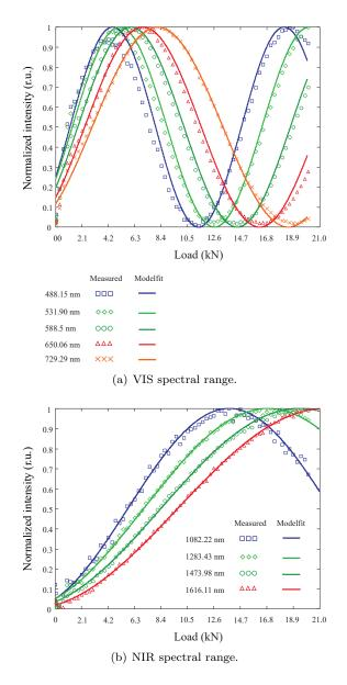
Fig. 6: Normalized intensity of light at the output of the polariscope for selected wavelengths in VIS and NIR spectral ranges as function of the applied load fitted by normalized intensity calculated according to Eq. (4).
