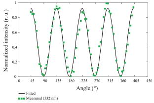
Fig. 3: Measured and calculated normalized intensity as function of rotation angle for wavelength  $\lambda = 532$  nm.
