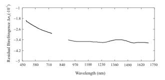
Fig. 4: Estimated wavelength dependence of the residual birefringence  $\Delta n_0$  of the investigated PMMA sample.
