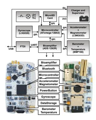
Fig. 2: ECG holter: Block diagram and PCB layout.
