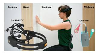
Fig. 1: Volunteer with wireless ECG holter on chest and EEG helmet Emotiv Epoc on head.
