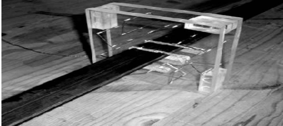
Fig.13. Rogowski coil coupled with the bar conductor in the position 1.
