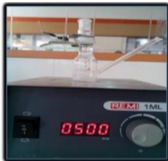
Figure No.2: Franz diffusion cell apparatus
