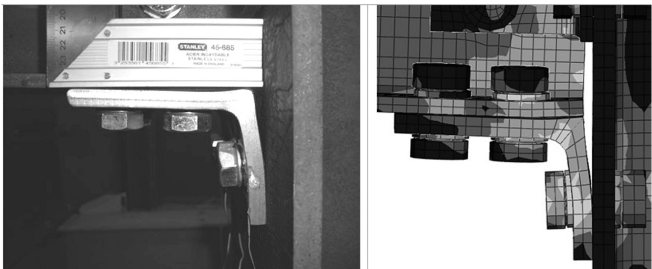
Figure 10. Comparative between test and FE model deformation behaviour in Test 1.
