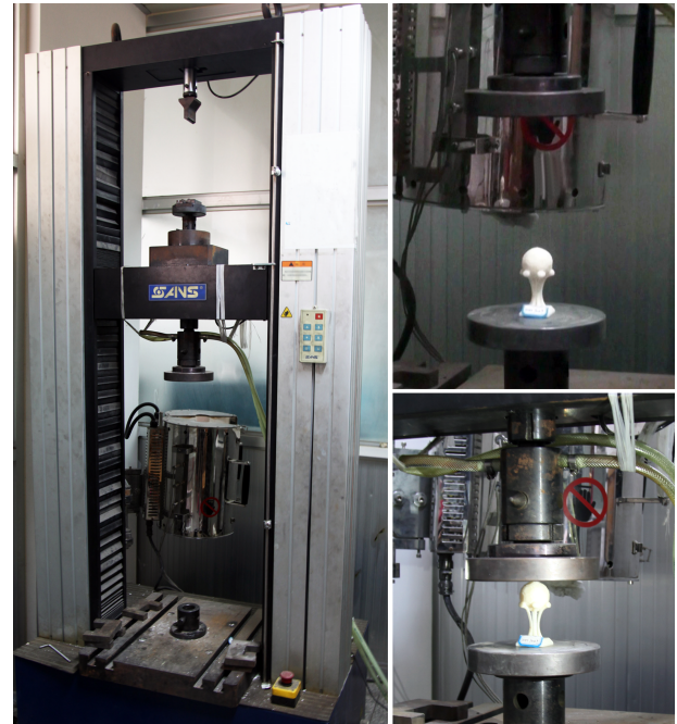
Figure 11: Compression tests using a universal testing machine.
