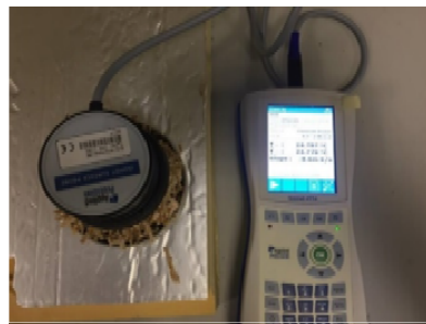
16 17 18 19 20 21 22 Figure 4. An image of saturated bio fibre thermal conductivity reading.
