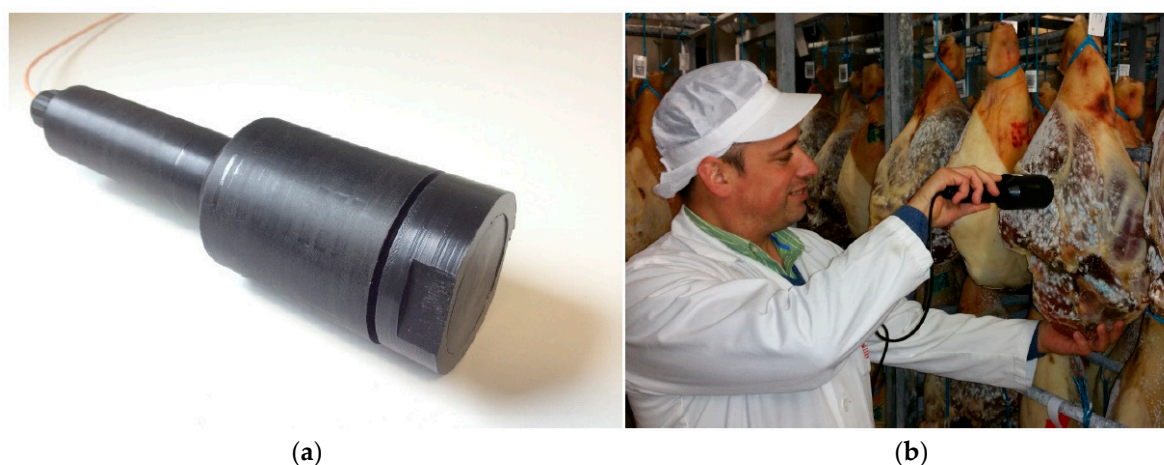
Figure 1. (a) The microwave probe and (b) the probe demonstrated at dry-cured production facility in Spain.
