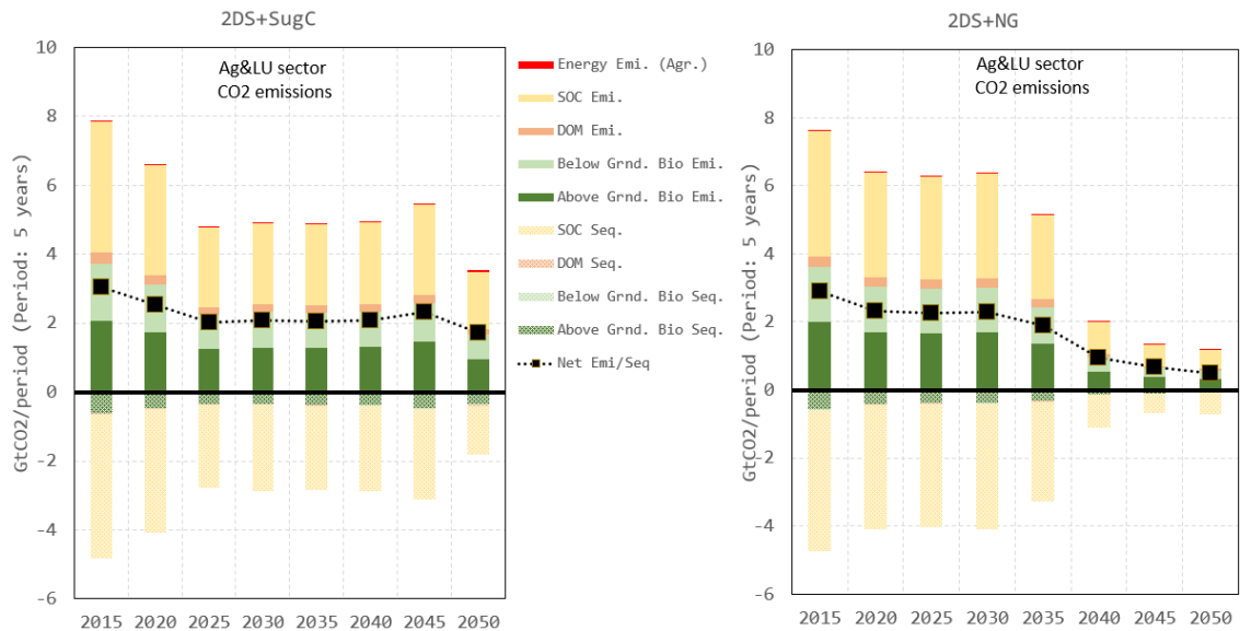
Figure 10. CO 2 emissions/sequestration rates from energy consumption in agriculture and land use dynamics
