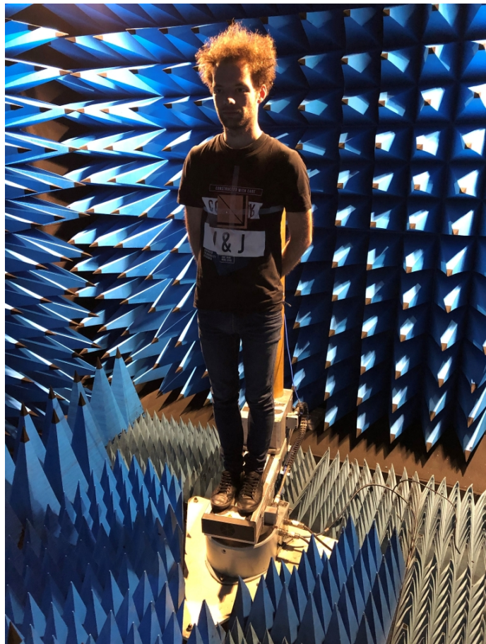
Fig. 2. Test person wearing the LoRa node in the anechoic chamber. Fully autonomous, no cables connected.
