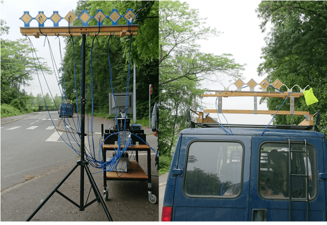
Fig. 1. Tx as a roadside unit (left) and Rx patch antennas on top of the van (right)
